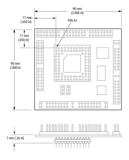
Figure 3–1: Dimensions of the PGA probe adapter
