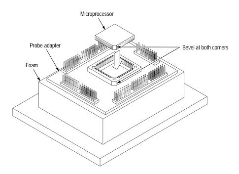
Figure 1-4: Placing a microprocessor into a PLCC probe adapter
