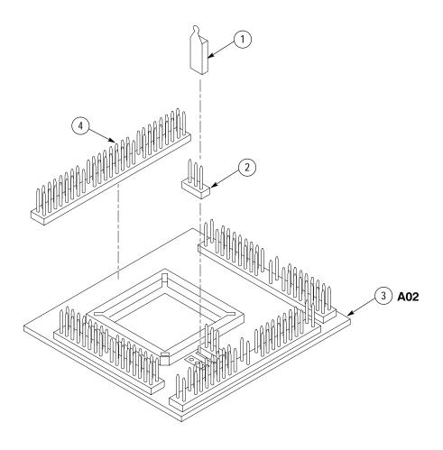
Figure 2: R3051, R3052 and R3081 probe adapter exploded view
