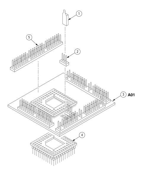
Figure 1: R3051, R3052 and R3081 probe adapter exploded view
