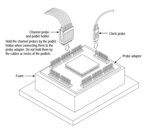
Figure 1–2: Connecting probes to a PGA probe adapter
