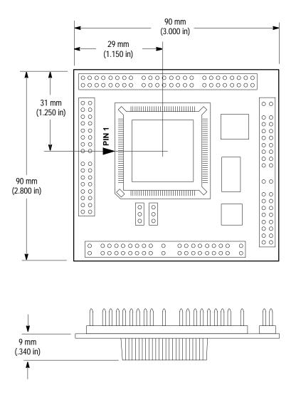
Figure 3–2: Dimensions of the probe adapter
