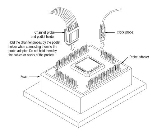
Figure 1–5: Connecting probes to a PLCC probe adapter
