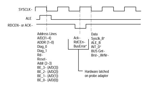
Figure 3-3: R3051, R3052 and R3081 bus timing with a probe adapter
