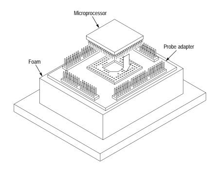
**6.** Place the microprocessor into the probe adapter as shown in Figure 1-1.
