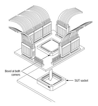
8. Place the probe adapter onto the SUT as shown in Figure 1–6.
